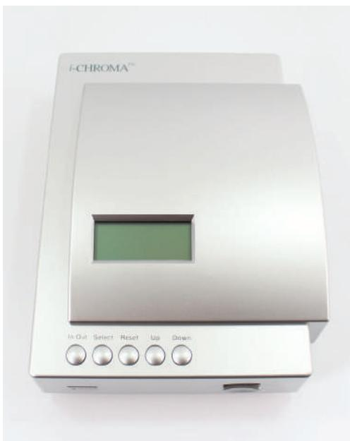
The ichroma™ reader is a first-generation portable fluorescent scanner that analyzes blood, urine, and other samples and displays measurement results on the screen. More than 30 immunoassay test cartridges can be measured using the ichroma™ reader.
